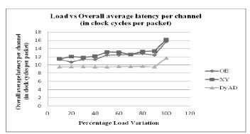
Figure5: Graph of Percentage Load variation vs Overall average latency per channel (in clock cycles per packet) for OE, XY and DyAD routing algorithm.
