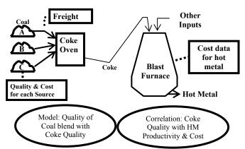
Figure 1: Schematic of hot metal production process
