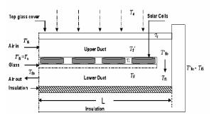
Figure 3(b): Schematic diagram of a hybrid photovoltaic thermal double pass air collector
