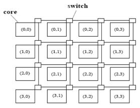
Figure 1: 4 X 4 2-Dimensional Mesh NoC
