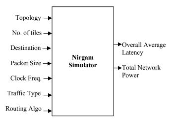
Figure3: Inputs and Outputs to Nirgam NoC Simulator
