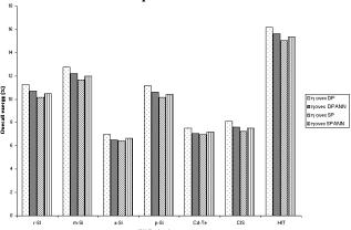
Figure 8: Annual variation of overall energy of single and double pass air collector of different PV technology
