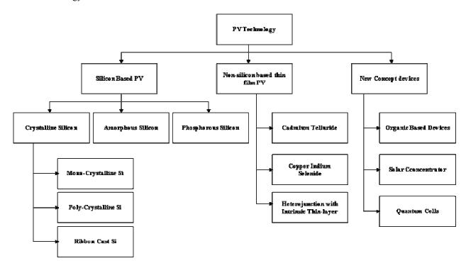
Table 1: Classification of photovoltaic on the basis of PV technology
