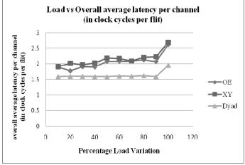
Figure 4: Graph of Percentage Load variation vs Overall average latency per channel (in clock cycles per flit) for OE,
