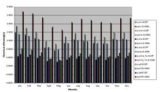
Figure 5(b): Monthly variation of electrical efficiency of double pass air collector for different PV technology
