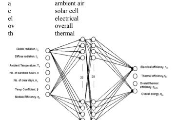
Figure 1(a): Input, output and hidden layers of ANN for single pass air collector
