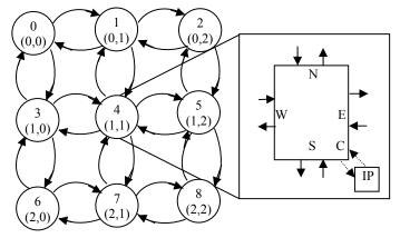
Figure 2: Architecture of a 2-dimensional 3x3 mesh topology based NoC
