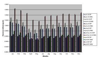
Figure 5 (a): Monthly variation of electrical efficiency of single pass air collector for different PV technology
